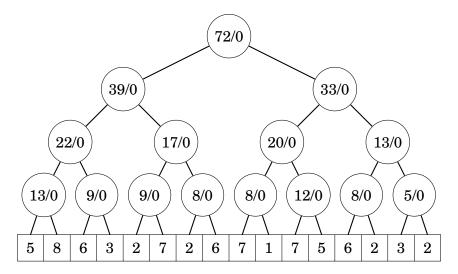
When the elements in [a,b] are increased by u, we walk from the root towards the leaves and modify the nodes in the tree as follows: If the range [x,y] of a node is completely inside the range [a,b], we increase the z value of the node by u and stop. If [x,y] only partially belongs to [a,b], we increase the s value of the node by hu, where h is the size of the intersection of [a,b] and [x,y], and continue our walk recursively in the tree.
