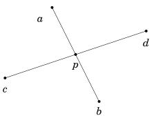
In this case, the line segments intersect exactly when both points c and d are on different sides of a line through a and b, and points a and b are on different sides of a line through c and d. Hence, we can use cross products to check this.
