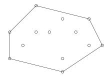
**Andrew's algorithm** [3] provides an easy way to construct the convex hull for a set of points in  $O(n \log n)$  time. The algorithm constructs the convex hull in two parts: first the upper hull and then the lower hull. Both parts are similar, so we can focus on constructing the upper hull.
