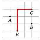
A useful technique related to Manhattan distances is to rotate all coordinates 45 degrees so that a point (x, y) becomes (x + y, y - x). For example, after rotating the above points, the result is:
