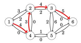
The minimum edge weight on this path is 3, so the path increases the flow by 3, and the total flow after processing the path is 5.
