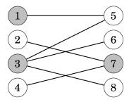
The nodes that do *not* belong to a minimum node cover form a **maximum independent set**. This is the largest possible set of nodes such that no two nodes in the set are connected with an edge. Once again, finding a maximum independent set in a general graph is a NP-hard problem, but in a bipartite graph we can use König's theorem to solve the problem efficiently. In the example graph, the maximum independent set is as follows:
