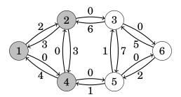
Now the minimum cut consists of the edges of the original graph that start at some node in A, end at some node outside A, and whose capacity is fully used in the maximum flow. In the above graph, such edges are  $2 \rightarrow 3$  and  $4 \rightarrow 5$ , that correspond to the minimum cut 6+1=7.
