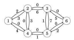
It is not possible to increase the flow anymore, because there is no path from the source to the sink with positive edge weights. Hence, the algorithm terminates and the maximum flow is 7.
