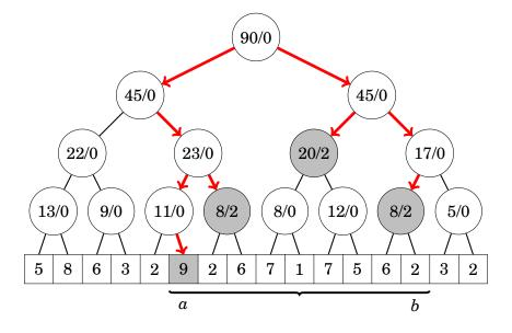
We also calculate the sum of elements in a range [a,b] by walking in the tree from top to bottom. If the range [x,y] of a node completely belongs to [a,b], we add the s value of the node to the sum. Otherwise, we continue the search recursively downwards in the tree.
