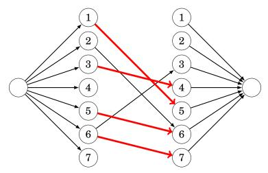
Each edge in the maximum matching of the matching graph corresponds to an edge in the minimum node-disjoint path cover of the original graph. Thus, the size of the minimum node-disjoint path cover is n-c, where n is the number of nodes in the original graph and c is the size of the maximum matching.
