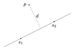
The area of the triangle whose vertices are  $s_1$ ,  $s_2$  and p can be calculated in two ways: it is both  $\frac{1}{2}|s_2-s_1|d$  and  $\frac{1}{2}((s_1-p)\times(s_2-p))$ . Thus, the shortest distance is
