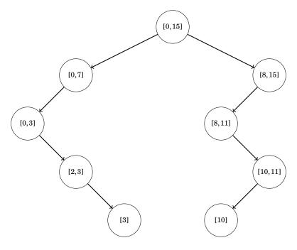
Any path from the root node to a leaf contains  $O(\log N)$  nodes, so each operation adds at most  $O(\log N)$  new nodes to the tree. Thus, after n operations, the tree contains at most  $O(n \log N)$  nodes.
