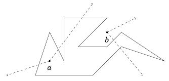
The rays from a touch 1 and 3 times the boundary of the polygon, so a is inside the polygon. Correspondingly, the rays from b touch 0 and 2 times the
