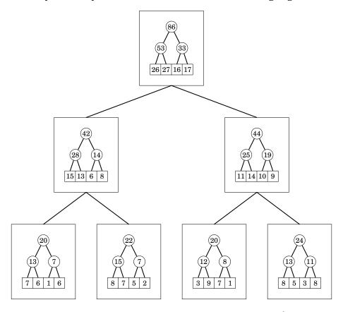
The operations in a two-dimensional segment tree take  $O(\log^2 n)$  time, because the big tree and each small tree consist of  $O(\log n)$  levels. The tree requires  $O(n^2)$  memory, because each small tree contains O(n) values.
