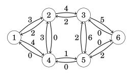
The idea is that increasing the flow decreases the amount of flow that can go through the edges in the future. On the other hand, it is possible to modify the flow later using the reverse edges of the graph if it turns out that it would be beneficial to route the flow in another way.
