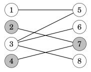
In this case, |X| = 2 and |f(X)| = 1, so the condition of Hall's theorem does not hold. This means that it is not possible to form a perfect matching in the graph. This result is not surprising, because we already know that the maximum matching of the graph is 3 and not 4.
