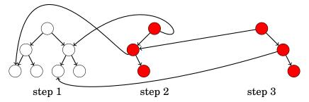
The structure of each previous tree can be reconstructed by following the pointers starting at the corresponding root node. Since each operation during the algorithm adds only  $O(\log N)$  new nodes to the tree, it is possible to store the full modification history of the tree.
