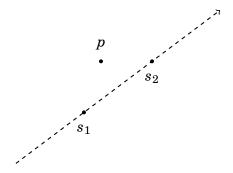
In this situation, the cross product  $(p-s_1) \times (p-s_2)$  tells us the location of the point p. If the cross product is positive, p is located on the left side, and if the cross product is negative, p is located on the right side. Finally, if the cross product is zero, points  $s_1$ ,  $s_2$  and p are on the same line.
