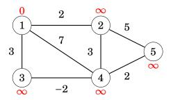
Each node in the graph is assigned a distance. Initially, the distance to the starting node is 0, and the distance to all other nodes is infinite.
