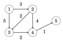
Now we can, for example, calculate the number of shortest paths from node 1 to node 5 using dynamic programming:
