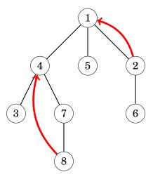
An easy way to calculate the value of f(x,k) is to perform a sequence of k moves in the tree. However, the time complexity of this method is O(n), because the tree may contain a chain of O(n) nodes.
