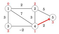
After this, no edge can reduce any distance. This means that the distances are final and we have successfully calculated the shortest distance from the starting node to all other nodes.
