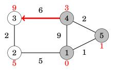
A remarkable property in Dijkstra's algorithm is that whenever a node is selected, its distance is final. For example, at this point of the algorithm, the distances 0, 1 and 3 are the final distances to nodes 1, 5 and 4.
