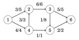
The notation v/k means that a flow of v units is routed through an edge whose capacity is k units. The size of the flow is 7, because the source sends 3 + 4 units of flow and the sink receives 5 + 2 units of flow. It is easy see that this flow is maximum, because the total capacity of the edges leading to the sink is 7.
