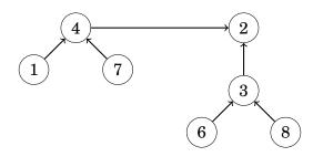
The resulting set contains the elements  $\{1,2,3,4,6,7,8\}$ . From this on, the element 2 is the representative for the entire set and the old representative 4 points to the element 2.
