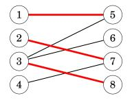
We can reduce the bipartite maximum matching problem to the maximum flow problem by adding two new nodes to the graph: a source and a sink. In addition, we add edges from the source to each left node and from each right node to the sink. After this, the maximum flow of the graph equals the maximum matching of the original graph.
