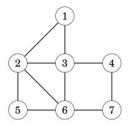
Suppose that the algorithm first creates a circuit that begins at node 1. A possible circuit is  $1 \rightarrow 2 \rightarrow 3 \rightarrow 1$ :
