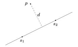
The area of the triangle whose vertices are  $s_1$ ,  $s_2$  and p can be calculated in two ways: it is both  $\frac{1}{2}|s_2 - s_1|d$  and  $\frac{1}{2}((s_1 - p) \times (s_2 - p))$ . Thus, the shortest distance is
