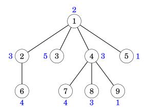
The idea is to construct a tree traversal array that contains three values for each node: the identifier of the node, the size of the subtree, and the value of the node. For example, the array for the above tree is as follows:
