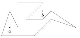
A convenient way to solve the problem is to send a ray from the point to an arbitrary direction and calculate the number of times it touches the boundary of the polygon. If the number is odd, the point is inside the polygon, and if the number is even, the point is outside the polygon.
