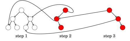
The structure of each previous tree can be reconstructed by following the pointers starting at the corresponding root node. Since each operation during the algorithm adds only  $O(\log N)$  new nodes to the tree, it is possible to store the full modification history of the tree.
