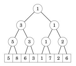
In this segment tree, every node in the tree contains the smallest element in the corresponding range of the array. The top node of the tree contains the smallest element in the whole array. The operations can be implemented like previously, but instead of sums, minima are calculated.
