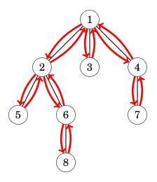
However, we use a bit different tree traversal array than before: we add each node to the array *always* when the depth-first search walks through the node, and not only at the first visit. Hence, a node that has k children appears k + 1 times in the array and there are a total of 2n - 1 nodes in the array.
