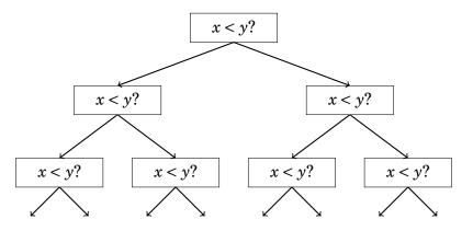
Here "x < y?" means that some elements x and y are compared. If x < y, the process continues to the left, and otherwise to the right. The results of the process are the possible ways to sort the array, a total of n! ways. For this reason, the height of the tree must be at least
