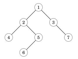
The nodes in a binary tree have three natural orderings that correspond to different ways to recursively traverse the tree:
