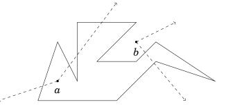
The rays from a touch 1 and 3 times the boundary of the polygon, so a is inside the polygon. Correspondingly, the rays from b touch 0 and 2 times the
