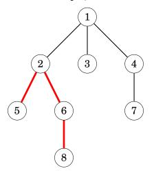
the lowest common ancestor of nodes 5 and 8 is node 2. A path from node 5 to node 8 first ascends from node 5 to node 2 and then descends from node 2 to node 8. The distances of the nodes from the root are d(5) = 3, d(8) = 4 and d(2) = 2, so the distance between nodes 5 and 8 is  $3 + 4 - 2 \cdot 2 = 3$ .
