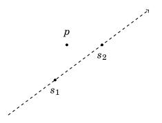
In this situation, the cross product  $(p - s_1) \times (p - s_2)$  tells us the location of the point p. If the cross product is positive, p is located on the left side, and if the cross product is negative, p is located on the right side. Finally, if the cross product is zero, points  $s_1$ ,  $s_2$  and p are on the same line.
