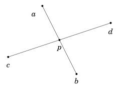
In this case, the line segments intersect exactly when both points c and d are on different sides of a line through a and b, and points a and b are on different sides of a line through c and d. Hence, we can use cross products to check this.
