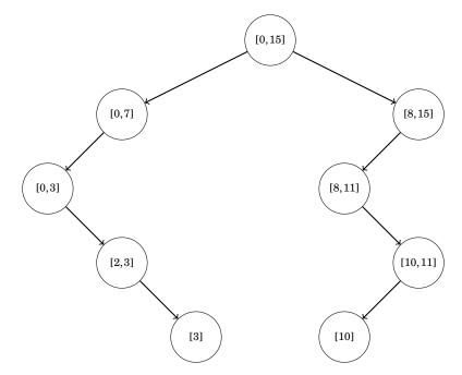
Any path from the root node to a leaf contains  $O(\log N)$  nodes, so each operation adds at most  $O(\log N)$  new nodes to the tree. Thus, after *n* operations, the tree contains at most  $O(n \log N)$  nodes.
