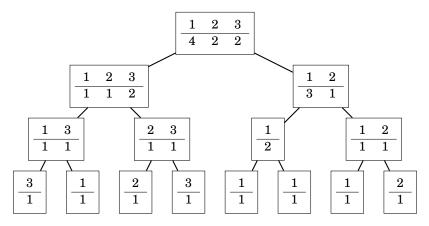
We can build the tree so that each node contains a map structure. In this case, the time needed for processing each node is  $O(\log n)$ , so the total time complexity of a query is  $O(\log^2 n)$ . The tree uses  $O(n \log n)$  memory, because there are  $O(\log n)$  levels and each level contains O(n) elements.
