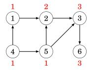
For example, since there are two paths from node 4 to node 2 and there is one path from node 4 to node 5, we can conclude that there are three paths from node 4 to node 3.
